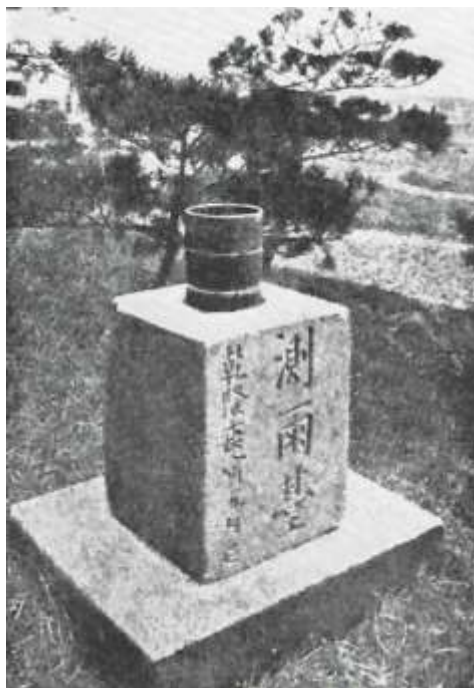
Figure 2. The rain gauge found at Taiku, 1770 A.D. (after Wada).
