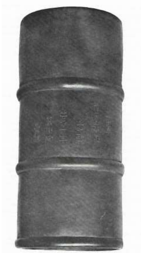
Figure 3. Plaster copy of an early Korean rain Gauge at the Science Museum, London (Crown copyright).
