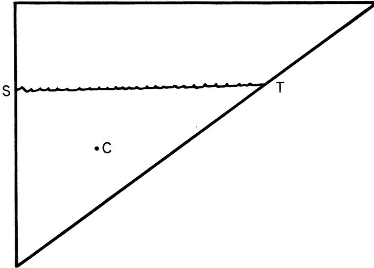
FIGURE 2. Here all the construction lines have been removed. Point C is the centre of gravity of the prism of water contained in the vessel when it has been filled to the elevation of S-T (the incipient point above which tipping will occur).
