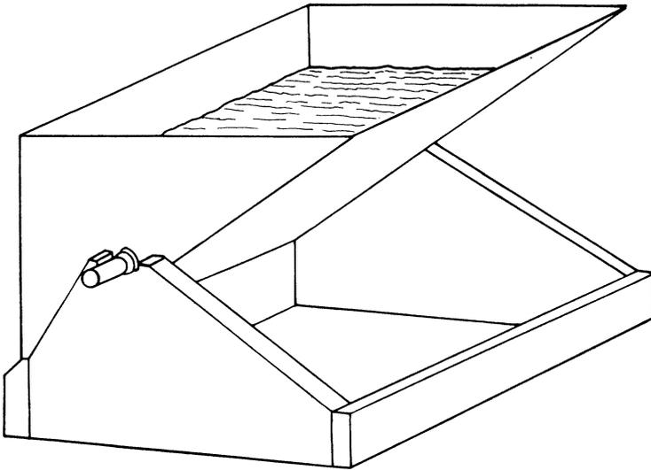
FIGURE 4. When assembled, Hooke's Tipping Bucket Rain-Gauge might have looked like this. Hooke mentioned that the vessel was 'Poiz'd like a balance upon a foot'. Maybe the 'Foot' was as shown above.
